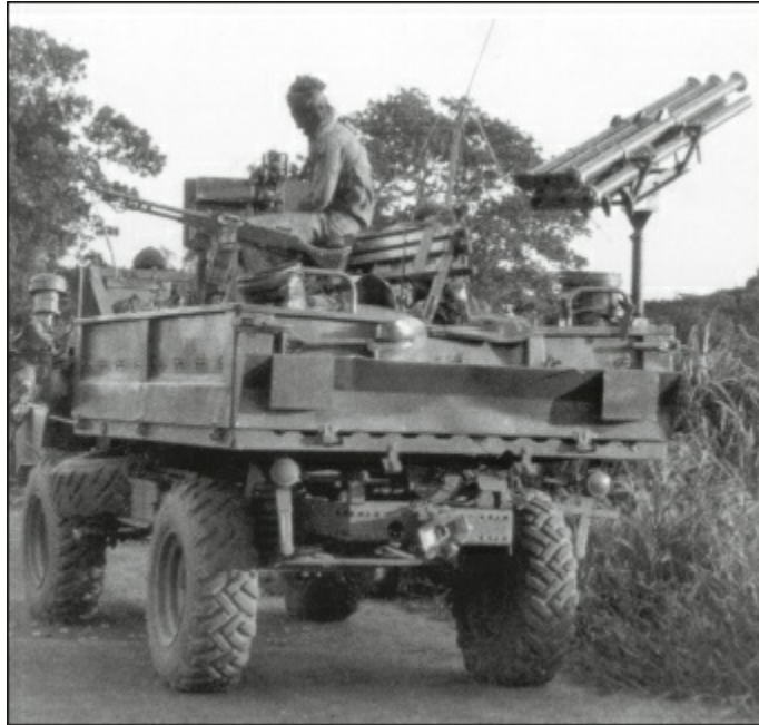
Unimog with home-made mounted SNEB and armour-piercing rocket launcher.
