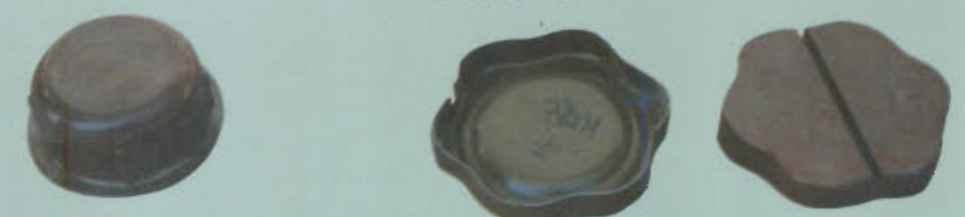
Fuse protection cap. Removed from MVZ 57 mechanism immediately prior to insertion in mine.
