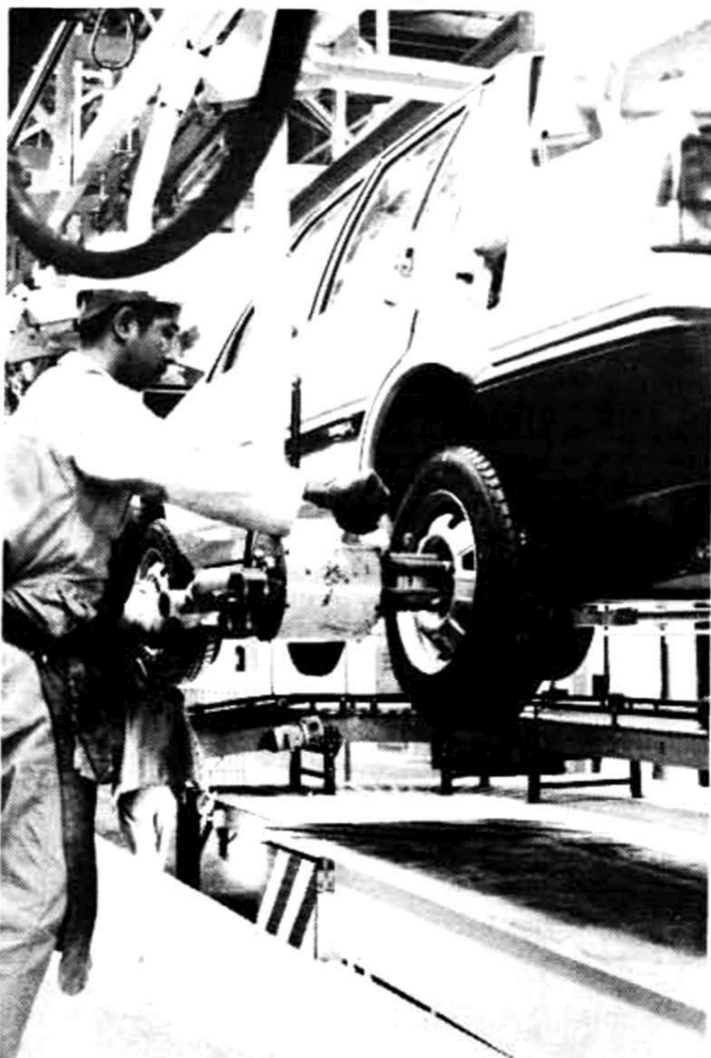
A worker on an assembly line tightens the wheel nuts A motor plant's body shop where the shell of the car is constructed
